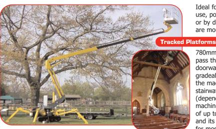
Ideal for both internal and external use, powered by an integral engine or by dc mains power. These units are mounted on a Mini-Excavator
