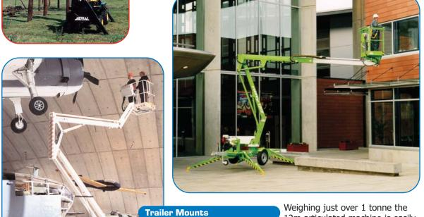
manoeuvred by one man. Telescopic retracting axles allow the machine to pass through 1.1m openings. Some 12m and 17m machines have an extra telescopic boom section and hydraulic outriggers. All units have pressure sensitive outriggers, dual fully proportional controls and emergency descent systems.
