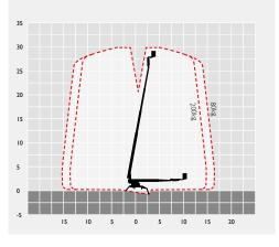
The information provided is for guidance only. It may change at any time in accordance with manufacturer's specification. Variable Jacking will affect working envelope. Outreach is variable depending on load, angle of rotation and outrigger configuration.
