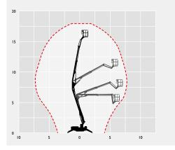
The information provided is for guidance only. It may change at any time in accordance with manufacturer's specification. Variable Jacking will affect working envelope. Outreach is variable depending on load, angle of rotation and outrigger configuration.
